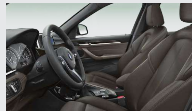
The Sport Seats for driver and front passenger are characterised by seat and backrest bolsters that are larger than those on the standard seats and, together with adjustable thigh support, for excellent ergonomics and better lateral support during fast cornering. In addition to the seat depth (mechanical), the backrest width (electric) can also be adjusted on the driver's seat.
